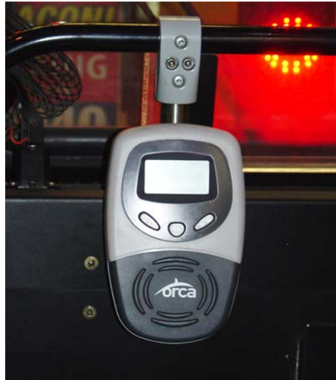
The ORCA On Board Fare Transaction Processor at left, installed and ready for action.
