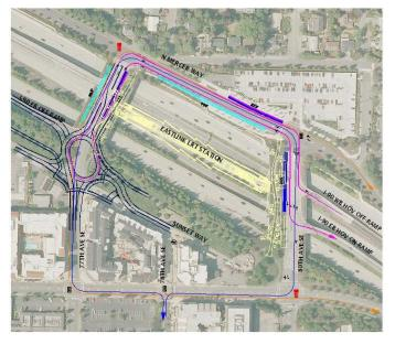
Scenario 4 represents a bus operating scheme that operates in a counter-clockwise direction from the westbound 80th Ave. HOV offramp to the 80th Ave. HOV on-ramp with a new roundabout at N Mercer Way & 77th Ave. SE.
