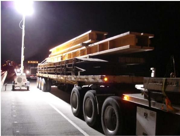
Static (stationary) load conditions were simulated by placing fully loaded test vehicles at specific locations on the bridge, followed by taking measurements. Dynamic (moving) load conditions then were simulated by driving the fully loaded test vehicles in train formation on the bridge's center roadway, with more measurements. Tests simulated single trains traveling in both directions along the bridge's length, and trains passing one another at mid-span and near the west end.
