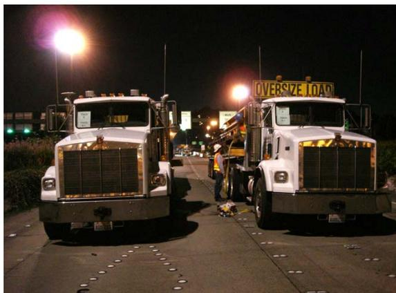
Traffic was shut down on the center roadway and westbound lanes during the night-time testing. The test involved eight flatbed trucks that were loaded to approximate the weight of light rail vehicles (148,000 pounds each, with two four-truck combinations each simulating a four-car light rail train).
