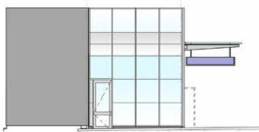
HEADHOUSE EAST ELEVATION
