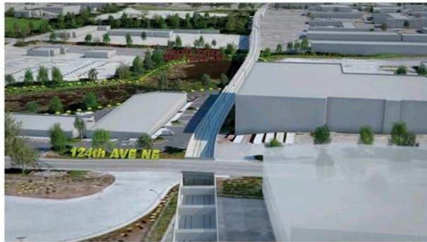
Retained cut under 124th Avenue NE, looking east (60% final design)
