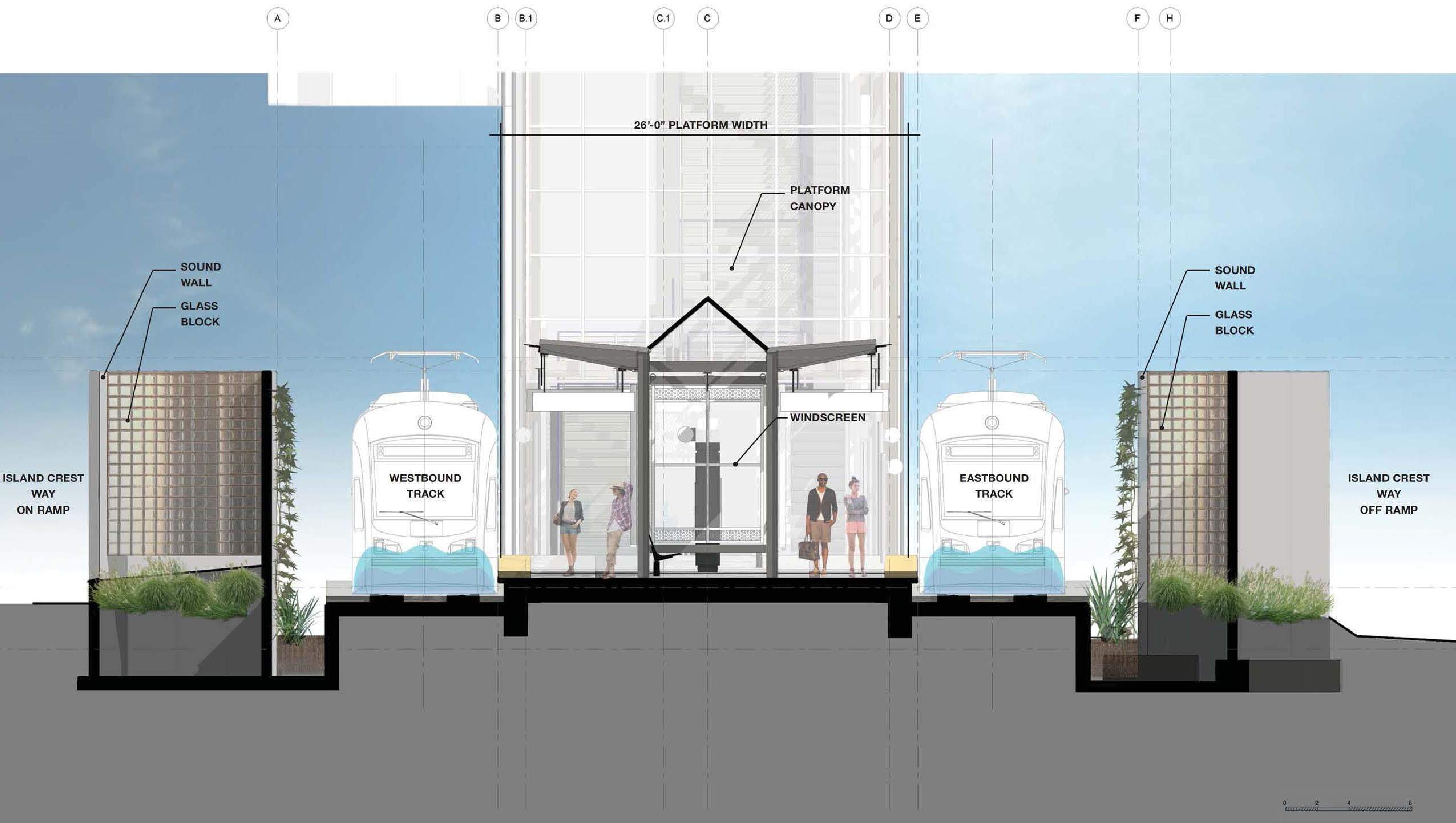
PLATFORM CROSS SECTION
