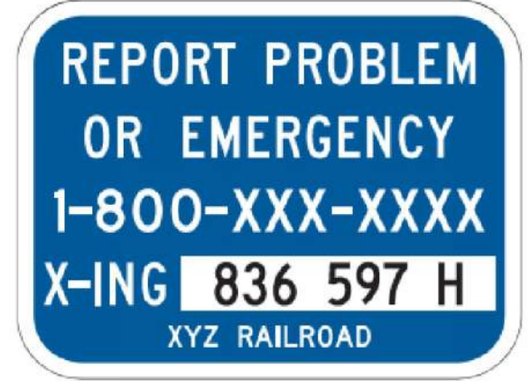
EXAMPLE OF EMERGENCY NOTIFICATION SIGN I13-1
