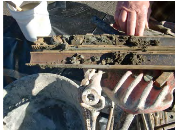
HC-20 sample contents at about 8 ft. below surface, fill material consisting of mixed and mottled sandy silts, including displaced glacial sediments.
