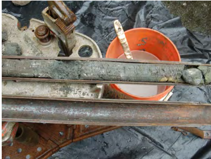
HC-3 sample contents at approximately 10 ft. below surface, illustrating redeposited glacial sediments.
