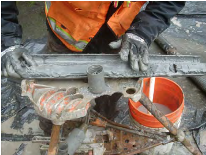
HC-3 sample contents at approximately 35 ft. below surface, glacial sediments consisting of very "clean", grey, clayey silts.
