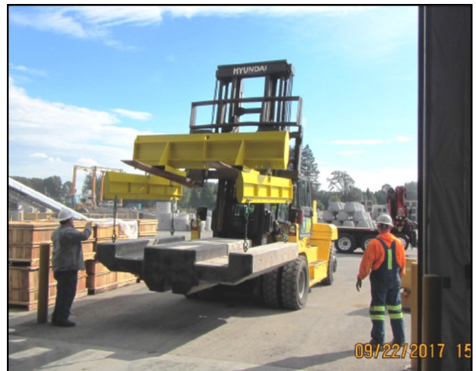
Columbia Precast: Transporting 7'-10" floating slab with new, larger forklift.
