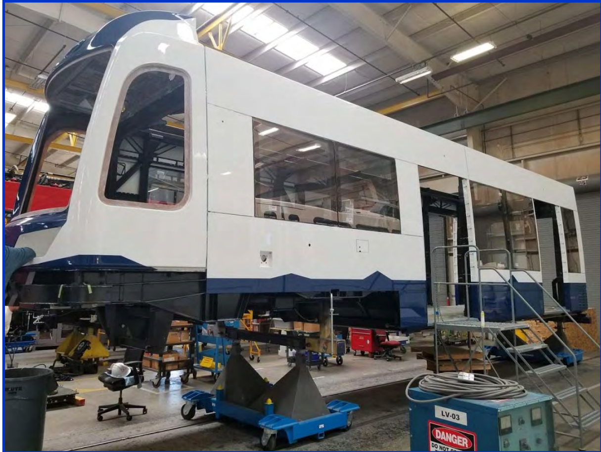
LRV Fleet Expansion– Car body painting is ongoing
