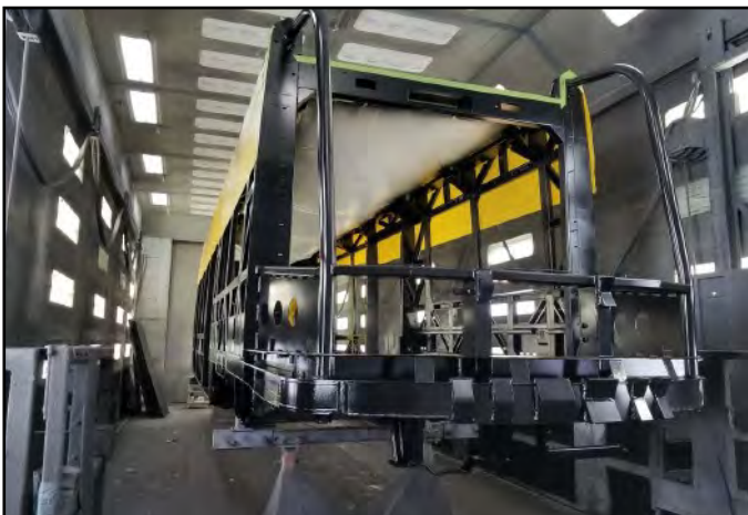
Primed Carbody getting baked in baking booth.
