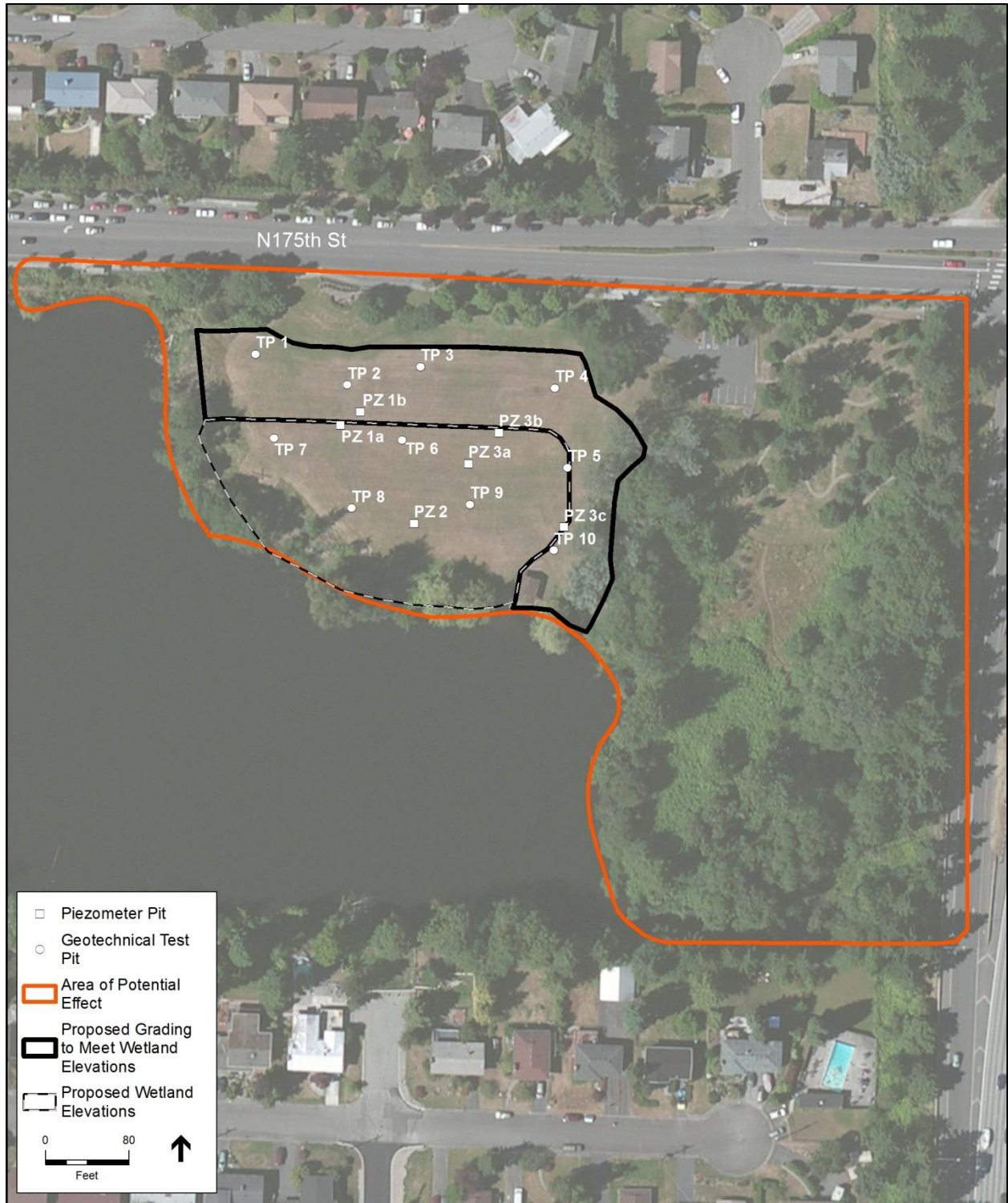
Figure 2 Location of subsurface geotechnical investigations for the Lynwood Link Ronald Bog Wetland Mitigation Project
