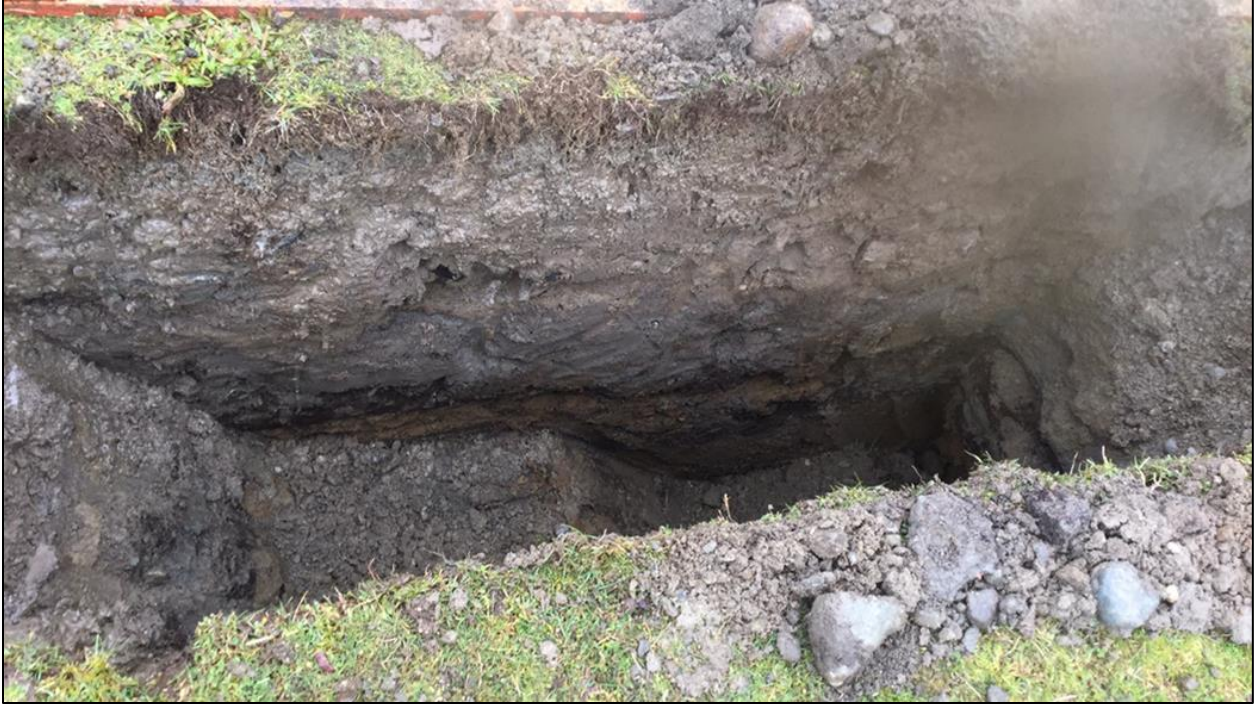
Figure 4 Overview of TP 2, grey material is imported fill, darker material is native silt.
