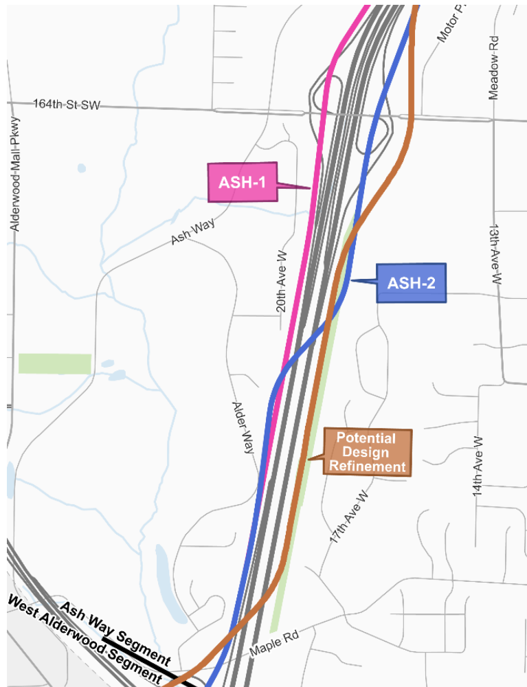
Figure 4-2 Potential Ash Way Guideway Shift
