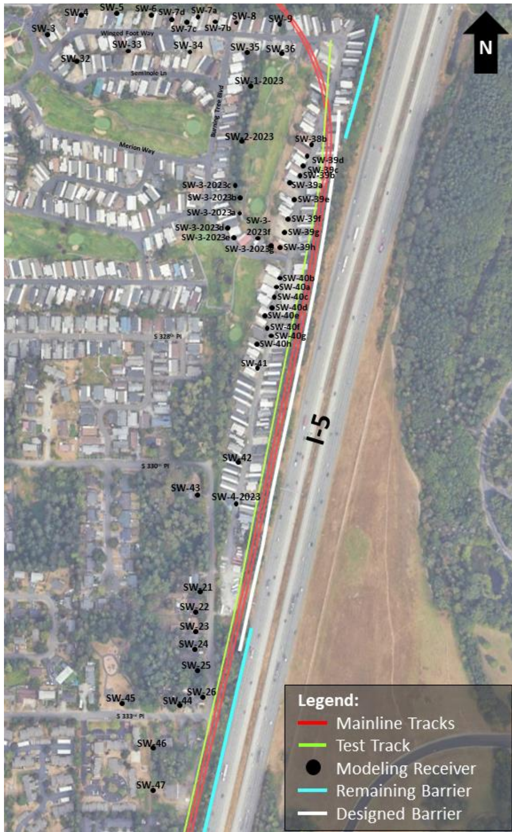
Figure 3. Designed wall to reduce noise levels below criteria
