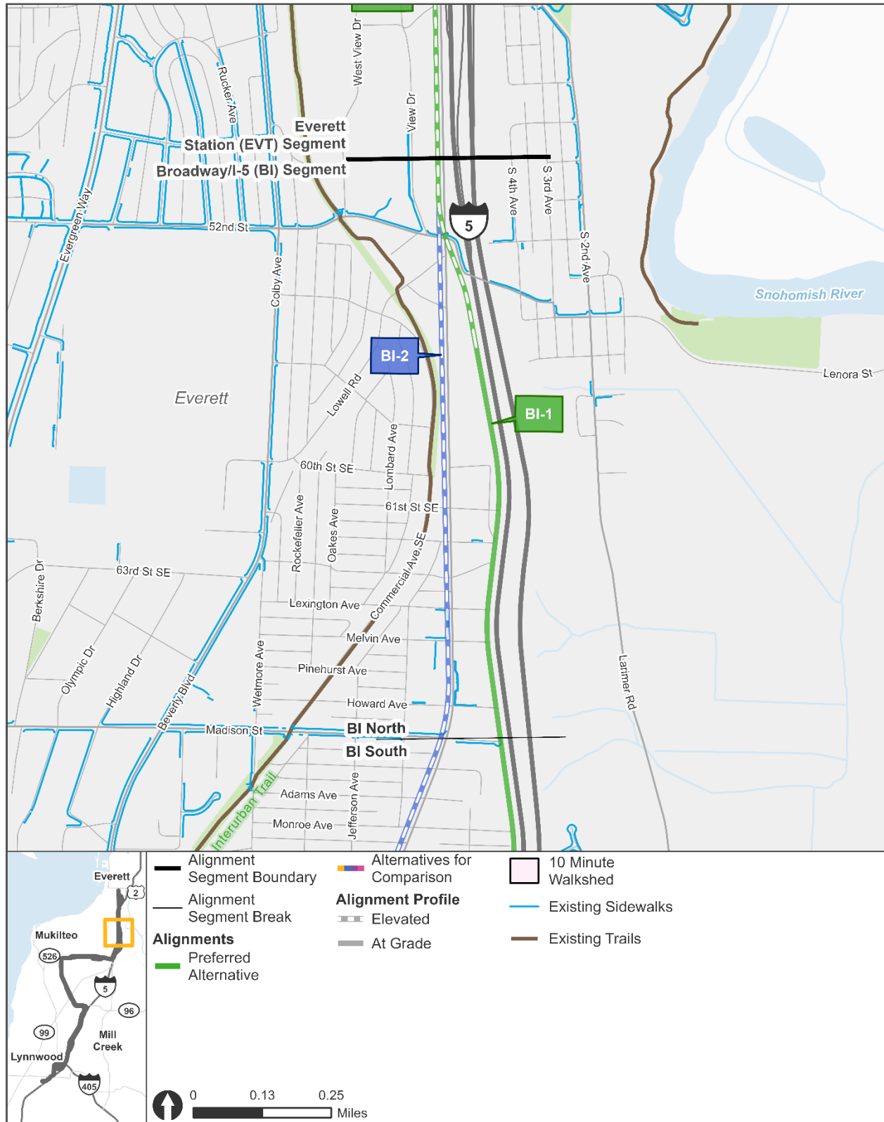
Figure 3-32 Existing Pedestrian Facilities – Broadway/I-5 Segment (North)
