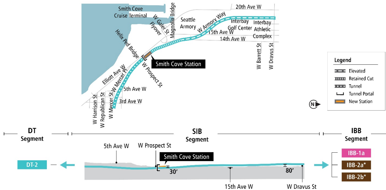
Figure 2-57. Plan and Profile for Prospect Street Station/Central Interbay Alternative (SIB-3)
