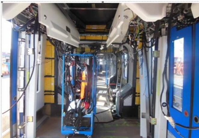
LRV #001 Hi-Pot Testing Interior of car.
