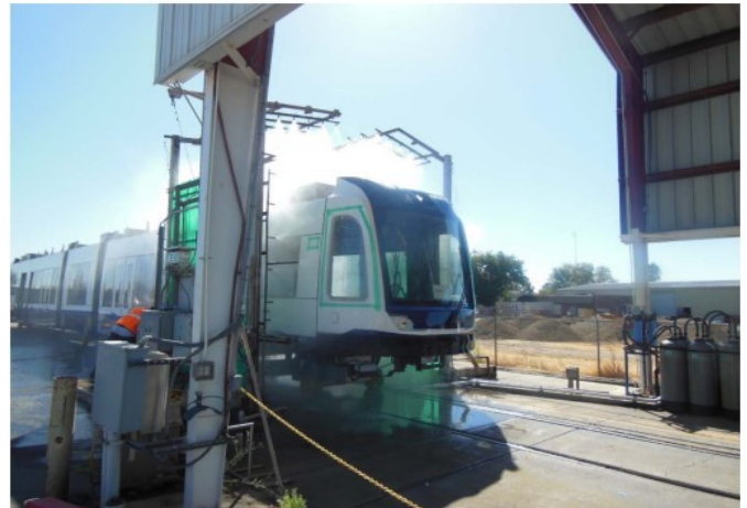
LRV #002 in Water Tightness Test.
