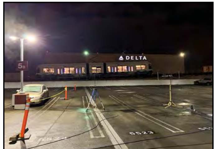
LRV 214 radiated emissions testing at Seattle, WA
