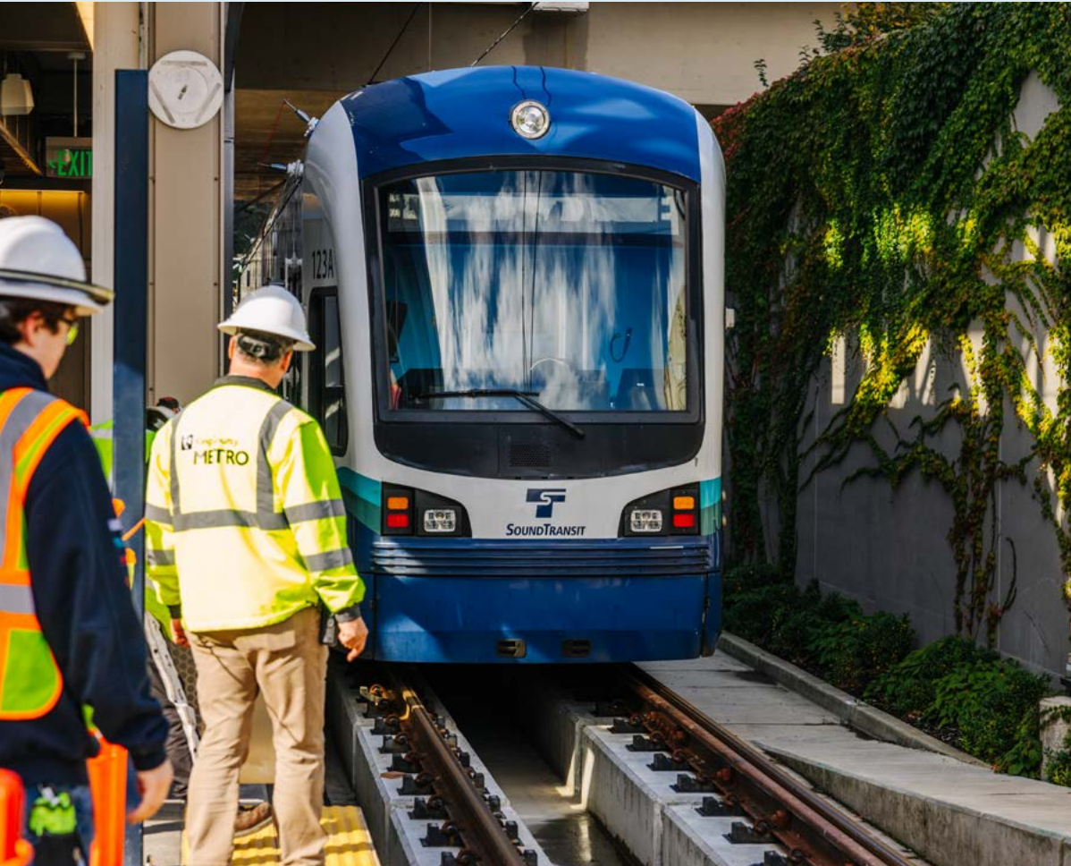
Workers perform “dead car pull” testing across the East Channel Bridge past the Mercer Island Station into the east approach of the Mercer Island tunnel.
