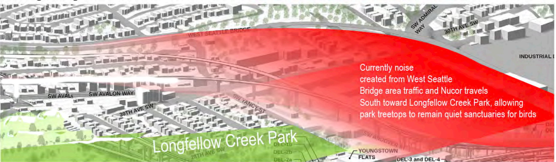
Delridge Segment Alternatives 3D Model Current Noise Pattern in Red
