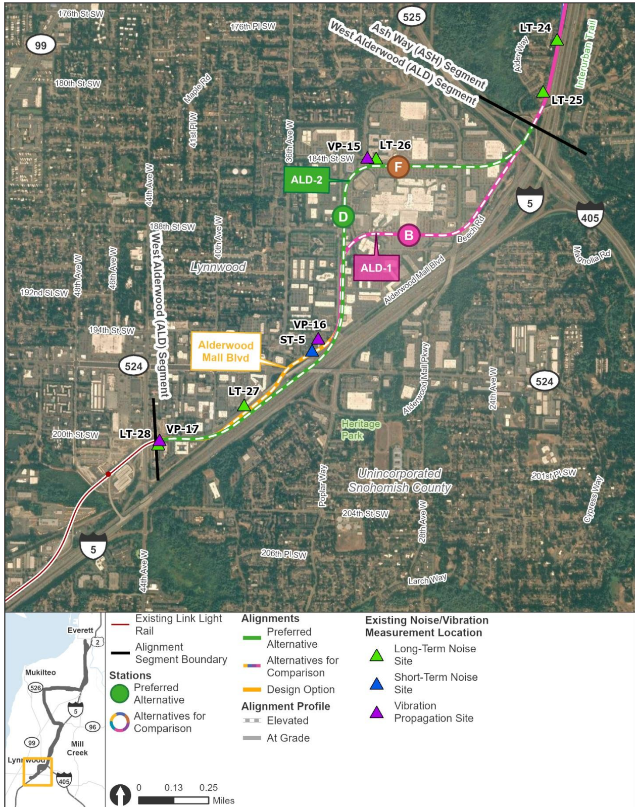
Figure 4-1 Existing Noise and Vibration Measurement Locations – West Alderwood Segment
