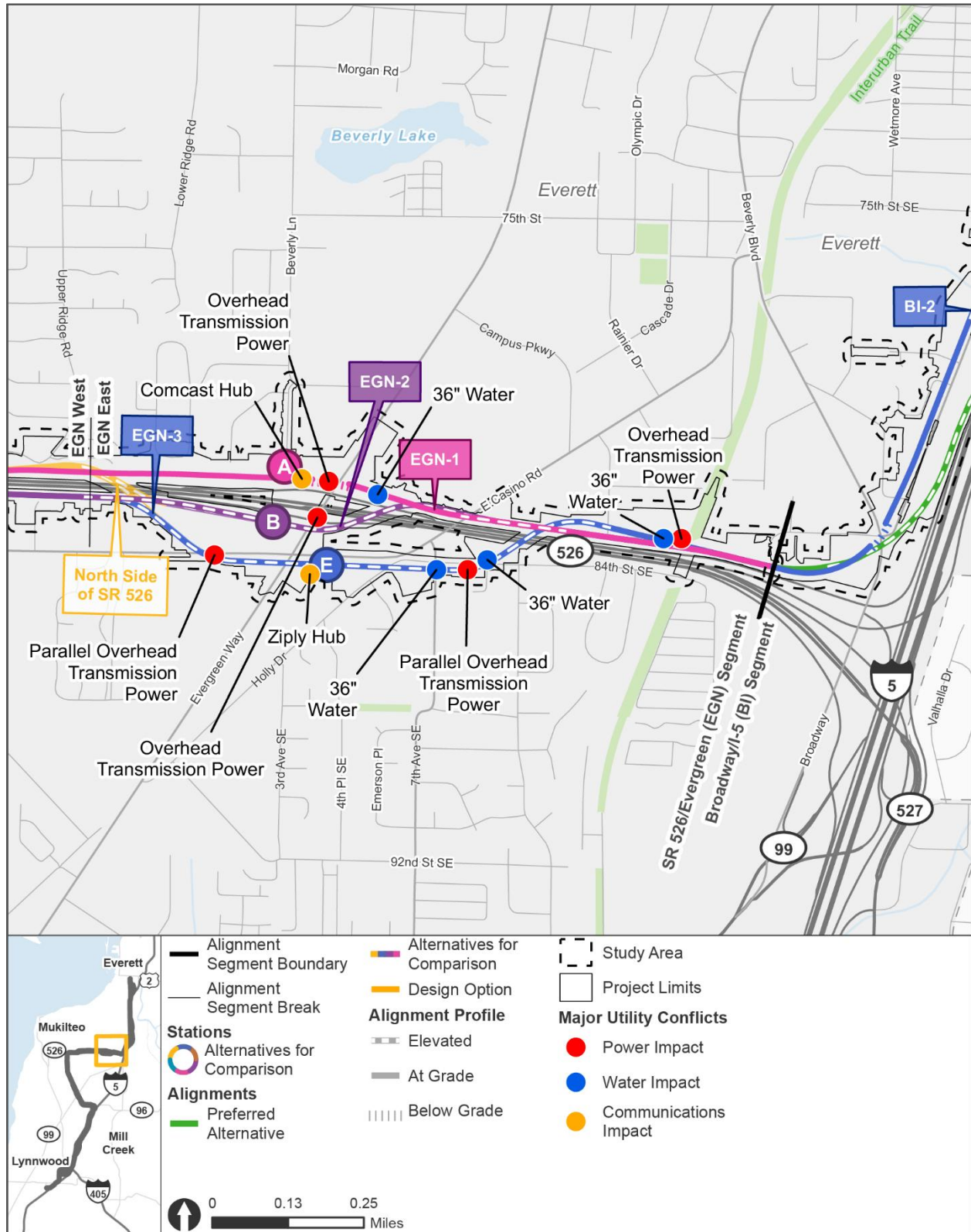
Figure 4-8 Major Utility Conflicts – SR 526/Evergreen Segment (East)
