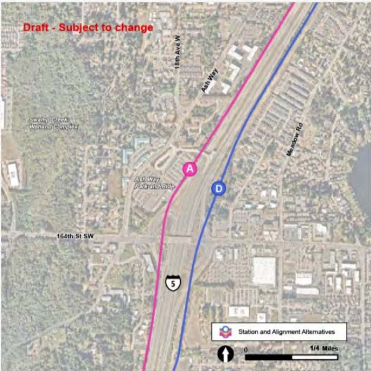
In this Ash Way station area map, the station alternatives are shown as options A and D, and route alternatives ASH-1 and ASH-2 are pictured in pink and blue, respectively. | Click on image to enlarge
