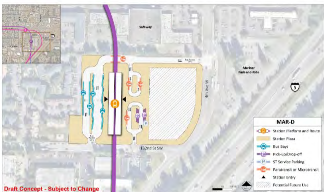
Early station layout for station alternative MAR-D, an elevated station between 4th Avenue W and 8th Avenue W across the street from Mariner Park-and-Ride. | Click on image to enlarge
