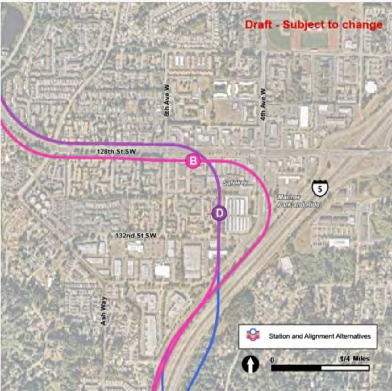
In this Mariner station area map, the station alternatives are shown as options B and D, and route alternatives MAR-1 and MAR-2 are pictured in pink and purple, respectively. | Click on image to enlarge
