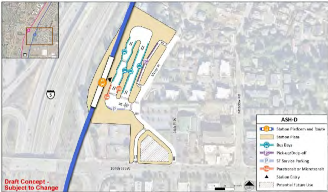
Early station layout for station alternative ASH-D, an elevated station located east of I-5 on 164th Street SW. | Click on image to enlarge
