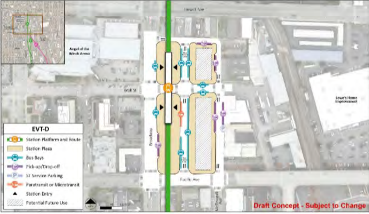
Early station layout for station alternative EVT-D, an elevated station located along Broadway just north of Pacific Avenue. | Click on image to enlarge
