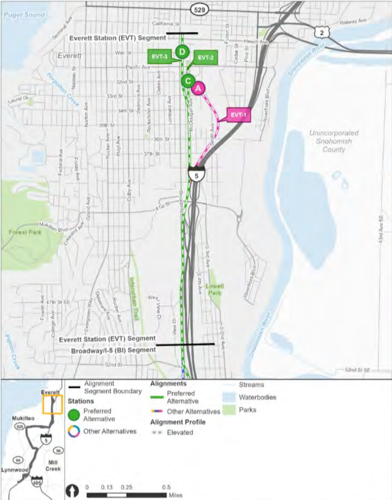
The Everett Station segment extends from the Broadway/I-5 segment to the project's end-of-line. Route alternatives EVT-1, EVT-2, and EVT-3 are pictured in pink and green, and the station alternatives are shown as options A, C, and D. | Click on image to enlarge
