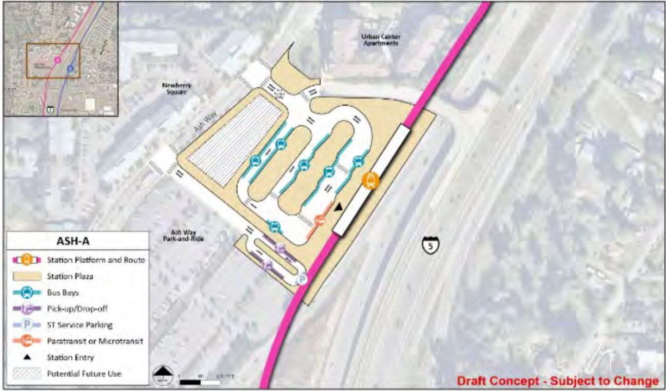
Early station layout for station alternative ASH-A, an elevated station on the west side of I-5 and adjacent to the Ash Way Park-and-Ride. | Click on image to enlarge
