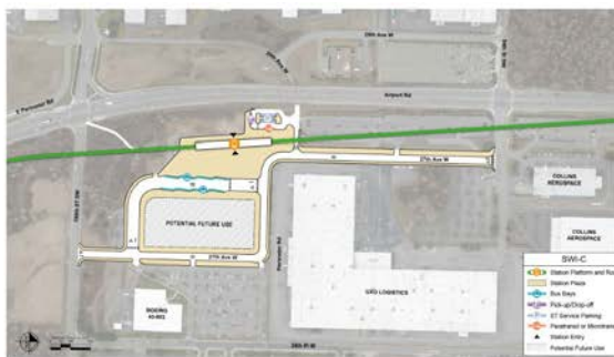
Updated station layout for station alternative SWI-C, an elevated station located along the northeast corner of Airport Road and 100th Street SW. | Click on image to enlarge
