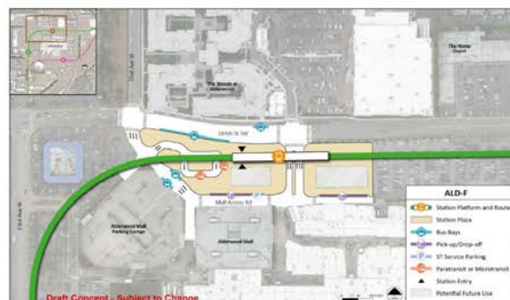
Early station layout for station alternative ALD-F, located on the north side of Alderwood Mall along 184th Street SW. | Click on image to enlarge
