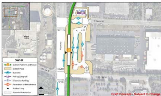
Early station layout for station alternative SWI-B, an elevated station located along the east side of Airport Road, south of Casino Road. | Click on image to enlarge
