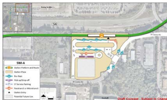
Early station layout for station alternative SWI-A, an elevated station located just south of SR 526 across the highway from Boeing. | Click on image to enlarge
