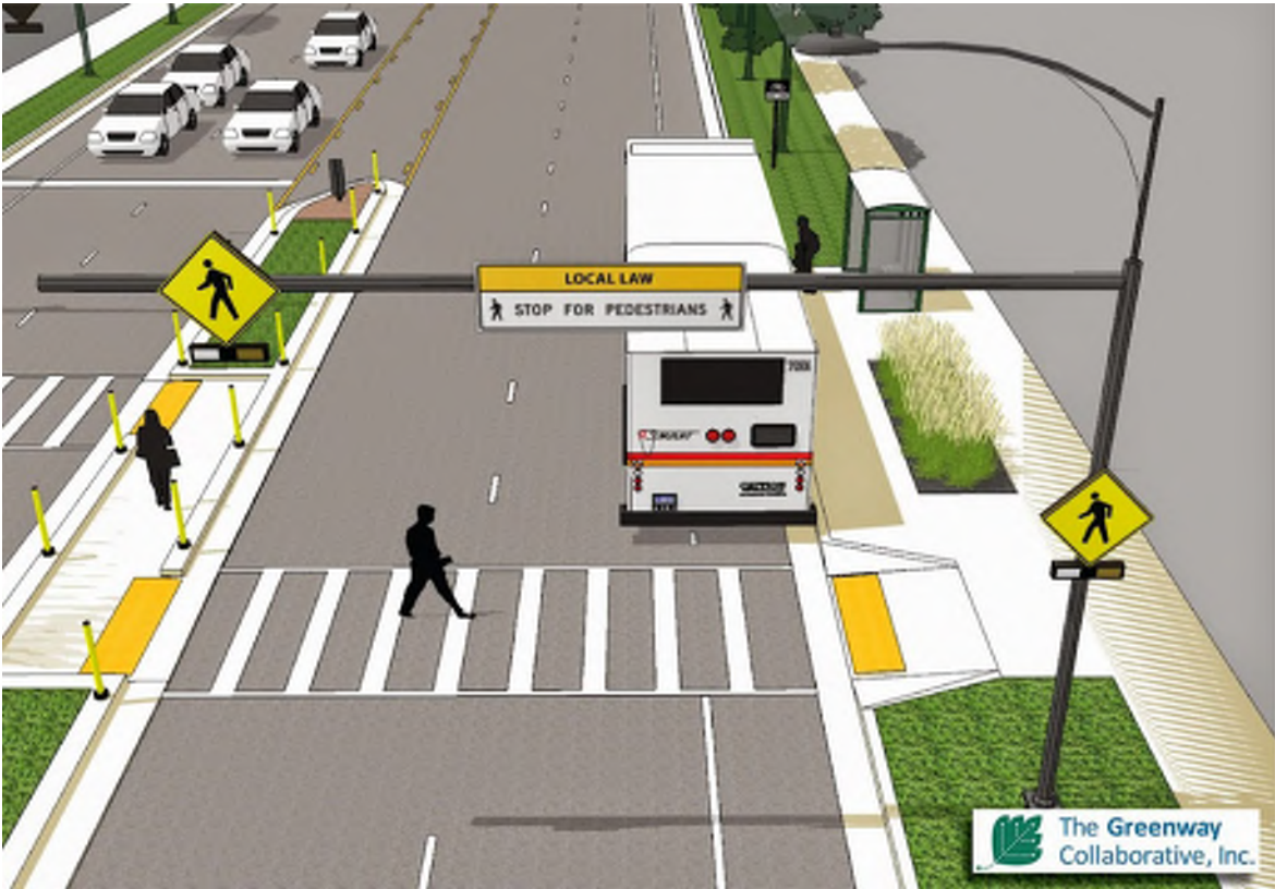
Figure 4-34 Staggered Crosswalks at a Z Crossing
