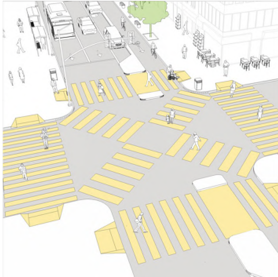
Figure 4-35 Pedestrian Scramble Design Example
