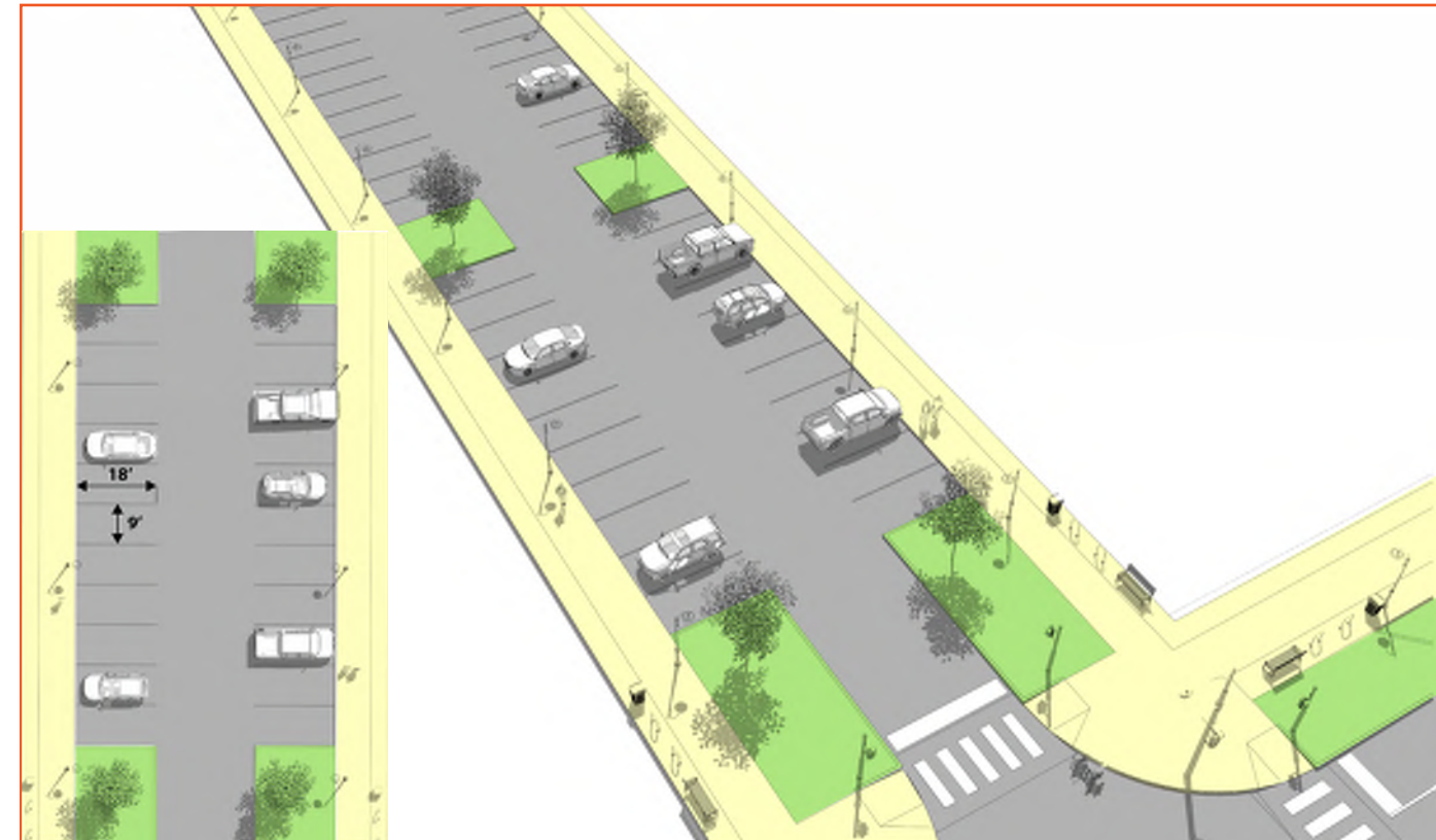
Figure 4-27 90 Degree Front-In Parking Example
