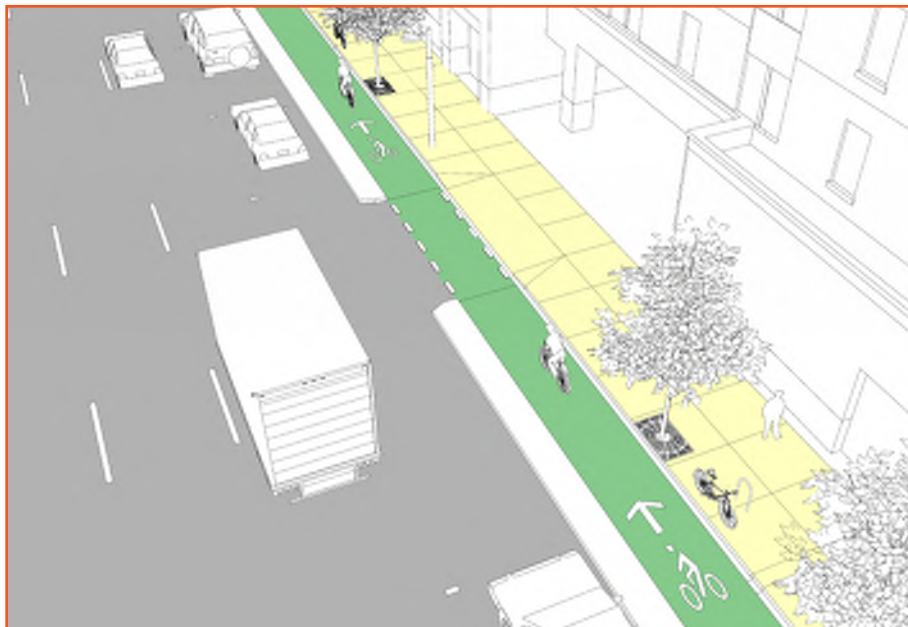
Figure 4-18 One-Way Cycle Track
