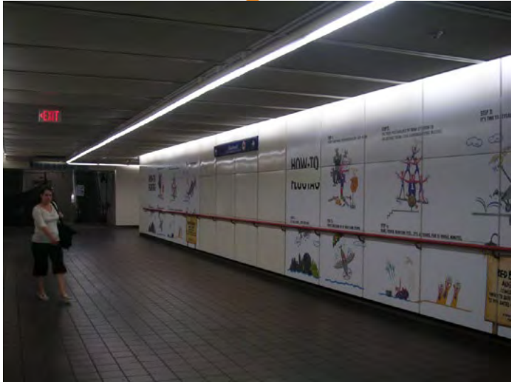
Horizontal Illuminance 8.6 fc Figure ii Granville Station, final passage to platform 2. Dark finishes, especially on the floors, can cause the space to be perceived as darker than it really is.
