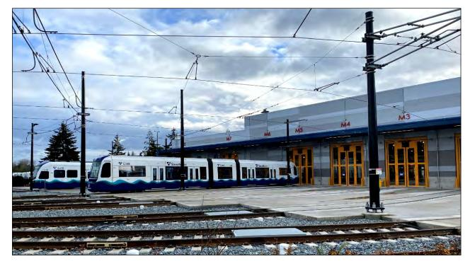
OMF East with LRVs from Kinkisharyo (at the back) and Siemens (in front)
