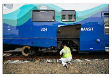
Brake pads are replaced on a Sounder Car
