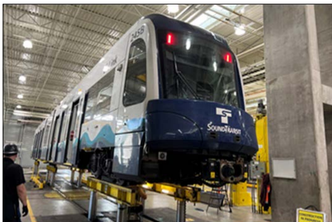
Car 245 slide plate replacement at Seattle, WA
