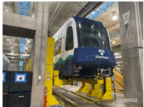
Car 282 wheel truing at OMF Central Seattle, WA
