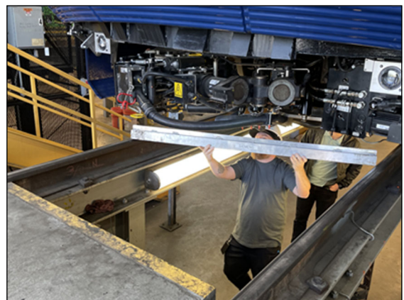
Car 280 Undercar Clearance Check in Seattle, WA
