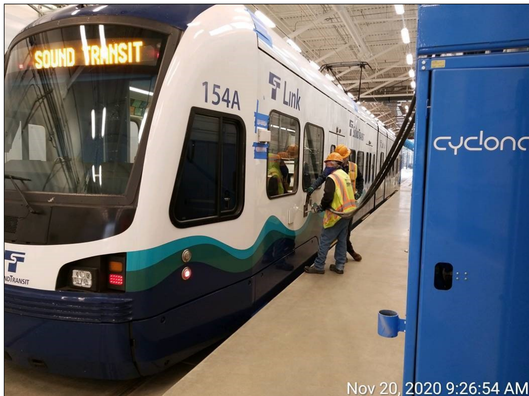
Kinkinsharyo Sandbos Fill—Sanding Equipment Commissioning Testing
