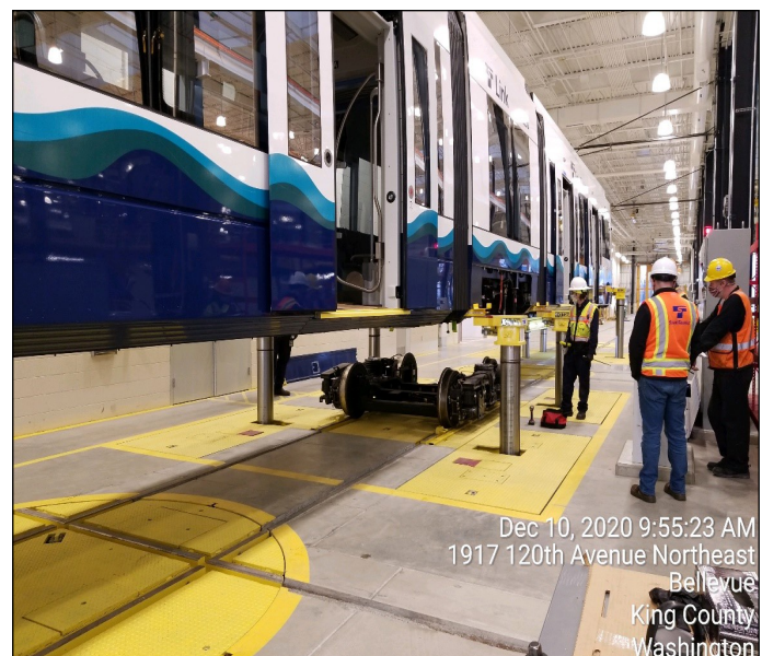
Siemens center wheel truck removal on track M7.
