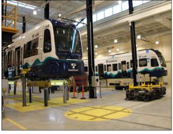
Kinkisharyo and Siemens LRVs lifted up by in-floor lift in the OMF Building.
