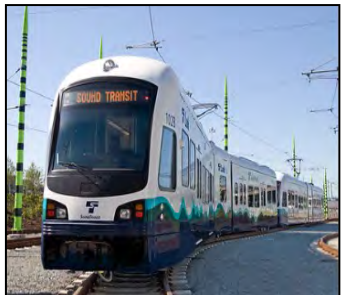
Light Rail Train run by the Overhead Catenary System (OCS) powered from the Traction Power Substation (TPSS).
