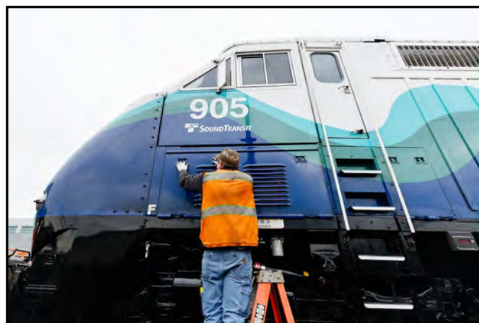
Air filters are changed at the Sounder maintenance base in Seattle
