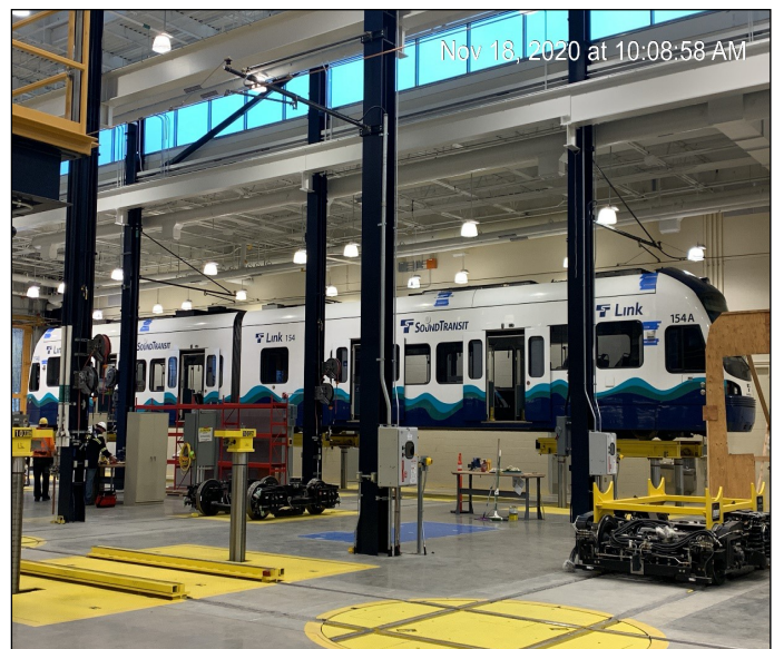
KI LRV on Lift Equipment for Equipment Commissioning.
