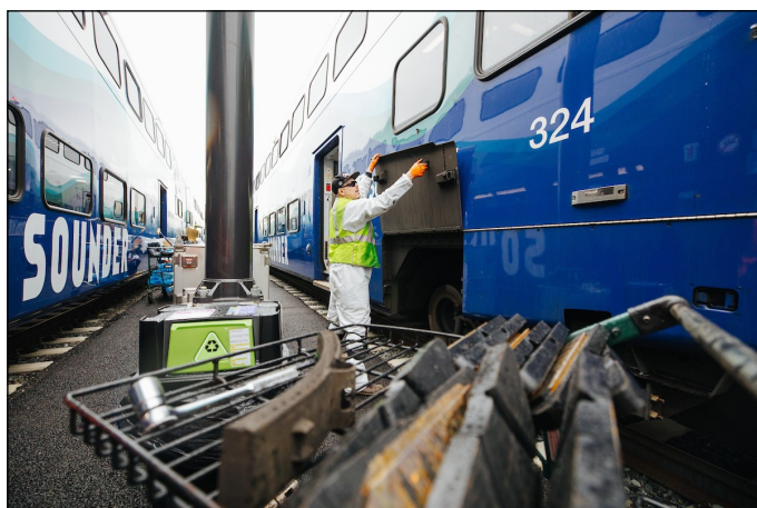
Brake pads are replaced on a Sounder car.
