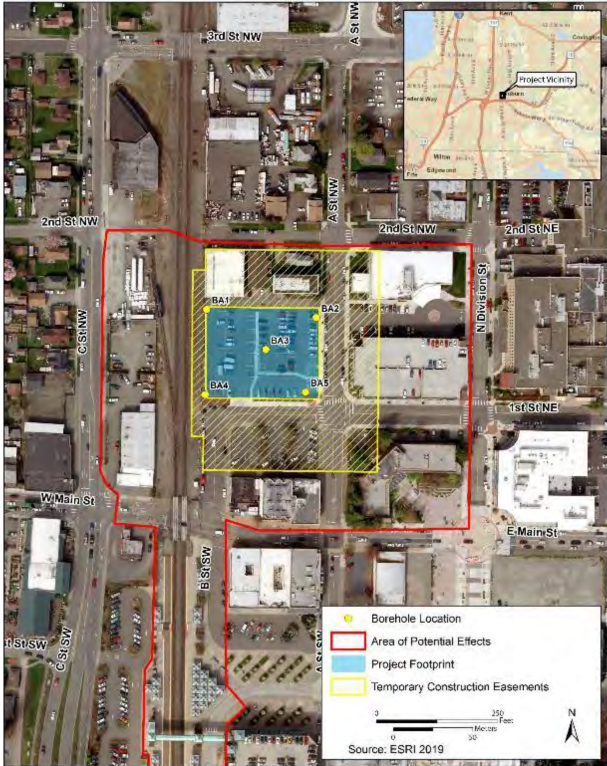
Figure 7-1 Geotechnical Borehole Locations
