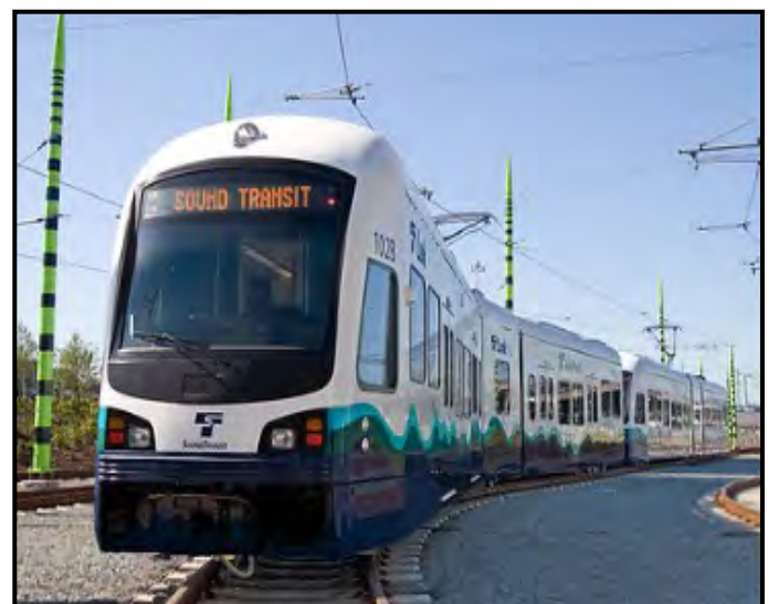
Light Rail Train run by the Overhead Catenary System (OCS) powered from the Traction Power Substation (TPSS).
