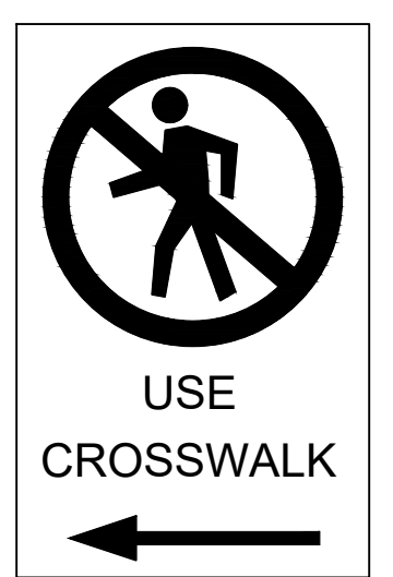
USE CROSSWALK LEFT R9-3B
