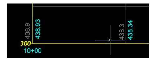
Set Profile View Band Styles at each major and minor station line to label existing ground elevation on the left and proposed grade elevation on the right.
