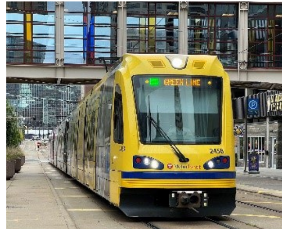
Figure: Wig Wag Train headlights as implemented by Metro Transit
