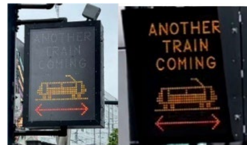
Figure: Example Another Train Coming signs
