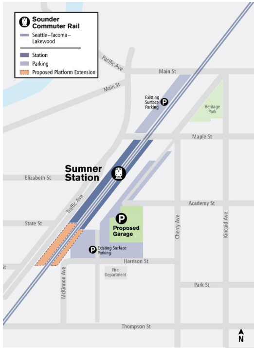
Figure 4-6 Sumner Station Proposed Platform Extension
