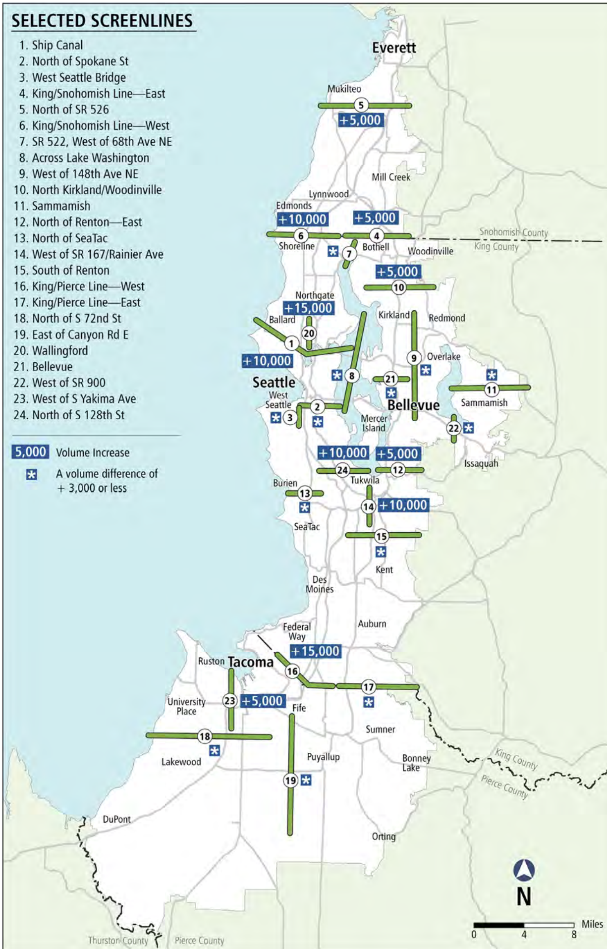
Figure 3-7. Daily transit ridership changes at selected screenlines—Current Plan Alternative vs. ST2
