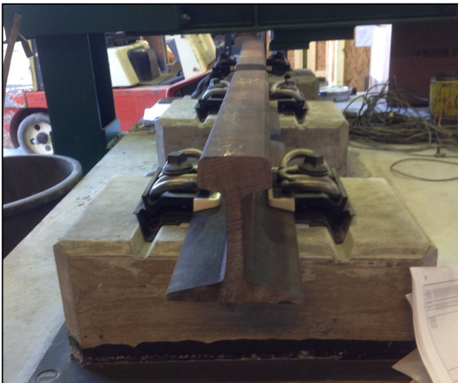
Plinth blocks ready for testing at the Structure Lab, University of Washington.
