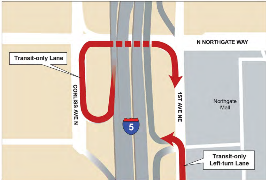
Figure 4-2. Northgate Area Transit Queue Bypass Improvement
