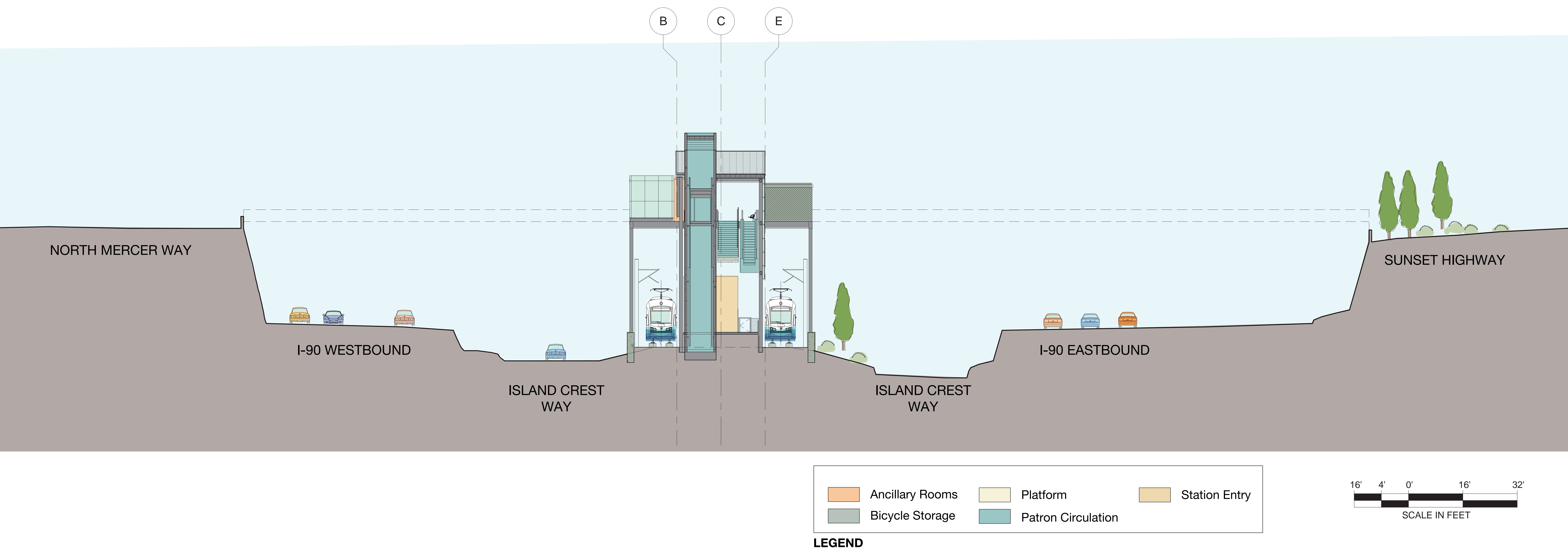
Site cross section C at east entry
