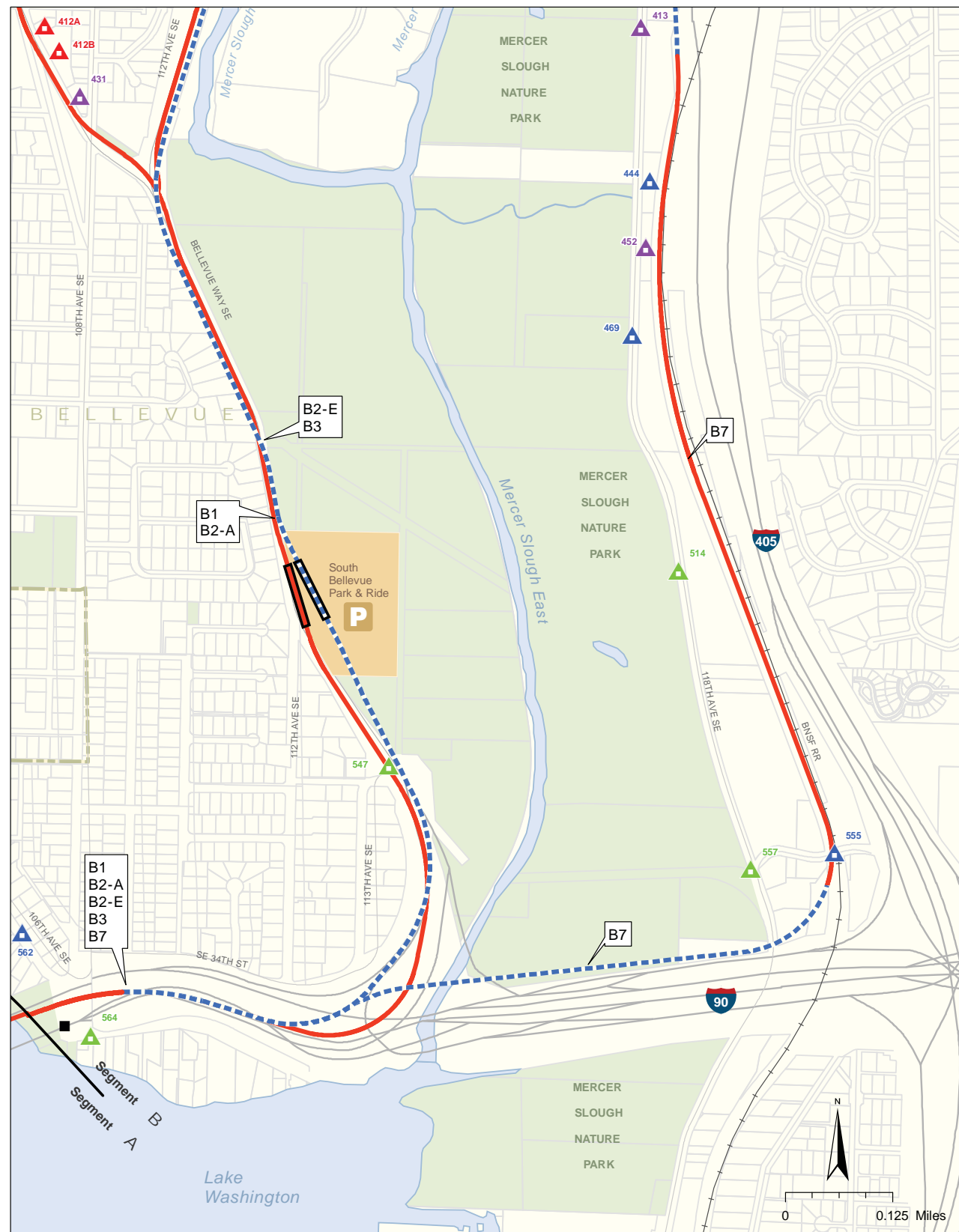
Hazardous Material Site Risk Levels ▲ High-Risk Site ▲ Medium-Risk Site ▲ Low-Risk Site ▲ Site with no Previous Release — Route At Grade - - - Elevated Route ···· Route in Retained Cut - - - Route in Tunnel ■ Traction Power Substation □ Proposed Station - - - City Limits Source: Data from Environmental Data Resources (2007) and King County (2006). Exhibit G3-5 Hazardous Material Sites Within 1/8 Mile of Alternatives Segment B East Link Project
