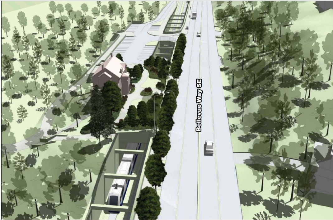
EXHIBIT A-1 Selected Alternative – B2M-C9T – Lidded trench in front of Winters House
