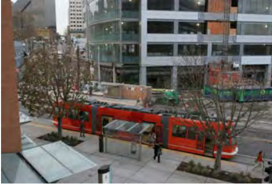
Figure 2 Typical Modern Streetcar Station Stop. Note seamless integration with sidewalk.
