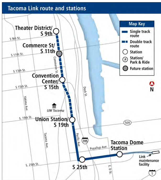
FIGURE 1-1 Existing Tacoma Link System
