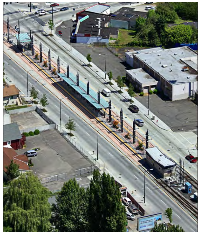
At-grade light rail station in median
