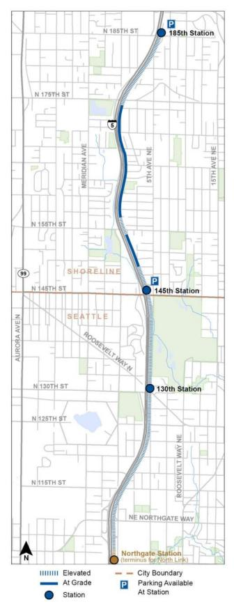
**Guideway:** The guideway runs along the east side of I-5, in WSDOT rights-of-way wherever possible, on elevated structure from Northgate Station to north of 145<sup>th</sup> Street, then retained cut/fill to 175<sup>th</sup> Street except for elevated crossings of 155<sup>th</sup> and 175<sup>th</sup> Street. North of 175<sup>th</sup> Street the guideway runs primarily on elevated structure to 185<sup>th</sup> Street.
