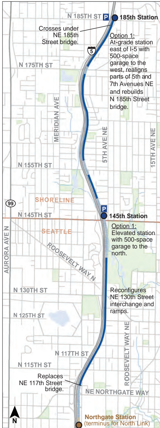
A1: AT-GRADE/ELEVATED TO NE 145th AND NE 185th STATIONS
